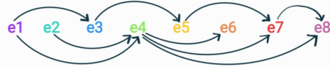
Fig. 5: Consumption order of EPs required in Example 1. A directed edge from e_i to e_j indicates e_i must be consumed before e_j .
