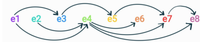
Fig. 5. Consumption order of EPs required in Example 1. A directed edge from e_i to e_j indicates e_i must be consumed before e_j .
